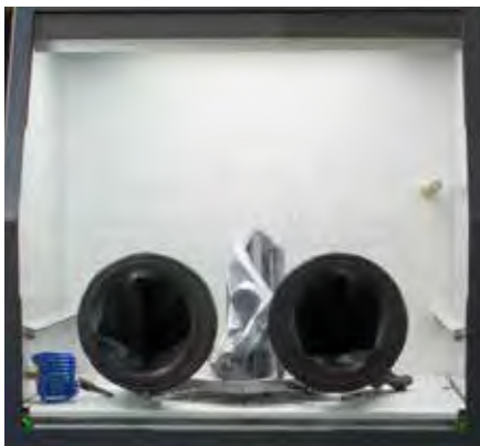
larger hand inlets improve ergonomics at the workplace
