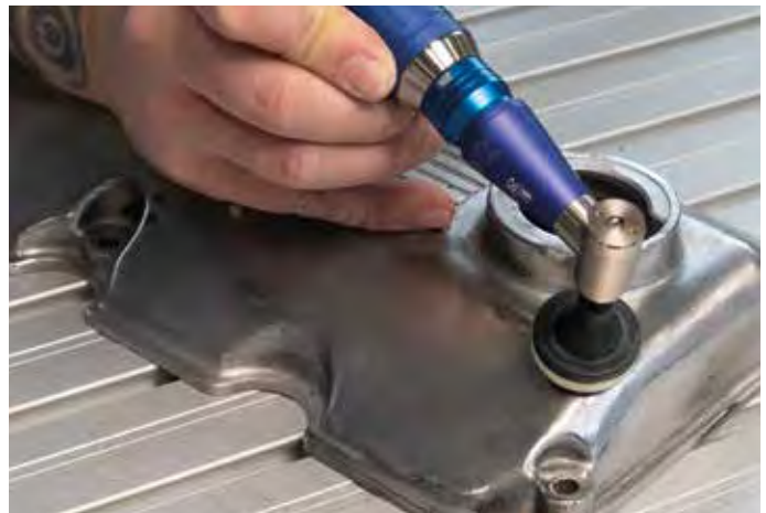
Aluminium polishing with angle-handpiece and felt
