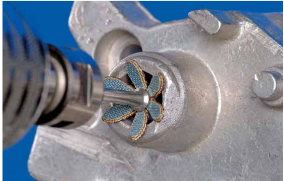
perfect for deburring of drill holes etc.
