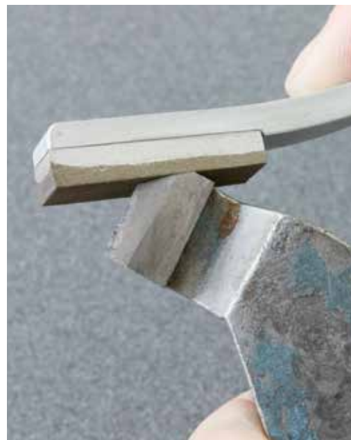
reworking of a carbide cutting edge with metal bond
